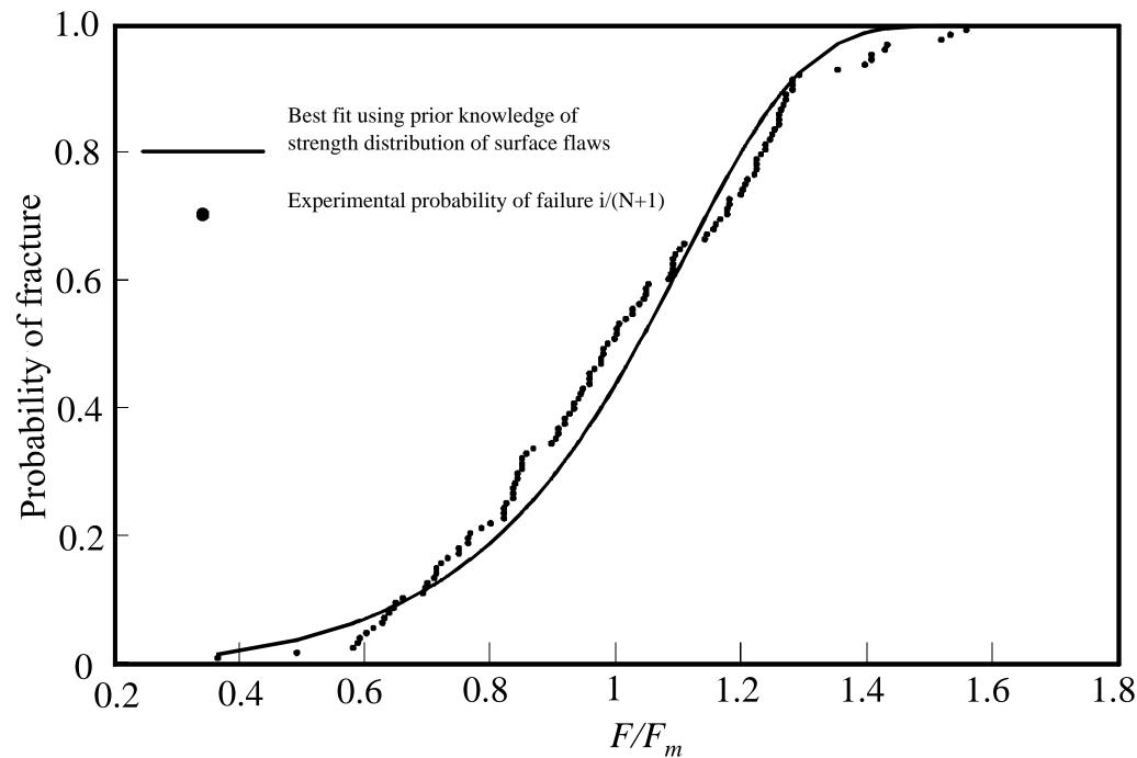
Fig. 5 The probability of fracture in the four-point-bend test
